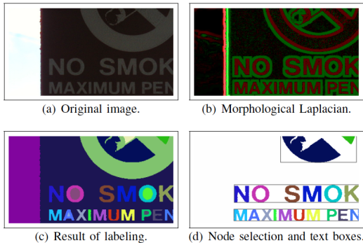
Fig. 27: Starting from a gray-level image (see (a)), we compute its well-composed gray-level Laplacian, then we deduce from its sign (see (b)) the labeling of the different characters (we look “inside” the zero-level-lines), and then we label the characters of the image (see (c) and (d)). This picture is extracted from [22].
