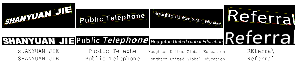
Figure 11: OCR recognition before and after the rectification process: original image (top), text rectification result (middle), OCR transcription before the rectification and OCR transcription after the rectification using Tesseract (bottom).
