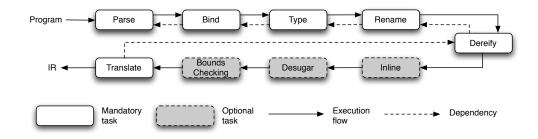
A compiler typically features three parts: the *front-end* analyzes the input program, the *middle-end* is independent of the source and target languages, and the *back-end* generates the output program in the target language. This figure focuses on the front-end.
