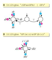
**Figure** 5.2: The translation offered for  $(\mathsf{GF}a \land \mathsf{GF}b) \lor \mathsf{GF}c$  is inferior to that given for the equivalent formula  $\mathsf{GF}(a \lor c) \land \mathsf{GF}(b \lor c)$ .
