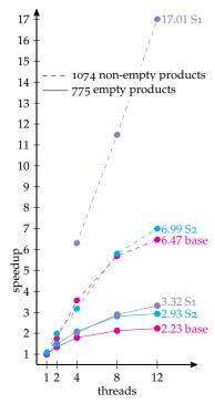
Figure 3.3: Speedups of running Dijkstra with 1, 2, 4, 8, and 12 threads (base). Without decomposition, or with decomposition using one of the two described strategies. All speedups are relative to Dijkstra with 1 thread, and averaged over 775 empty products (plain lines) or 1074 non-empty product (dashed lines).
