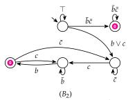
**Figure** 2.15: Automata for  $\varphi = F(Ga \lor (GFb \leftrightarrow GFc))$ . Automaton  $B_2$  is a simplified version of  $B_1$  assuming that a, b and c are mutually exclusive.
