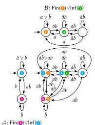
**Figure** 4.4: Depending on how we define the acceptance condition of the synchronous product of  $\mathcal{A}$  and  $\mathcal{B}$  we can intersect or merge their languages.
