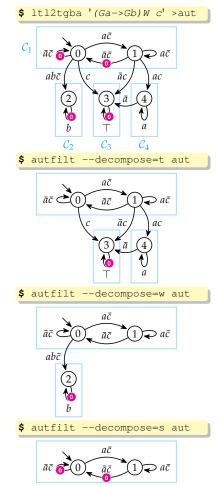
**Figure** 3.1: Decomposition of  $(Ga \rightarrow Gb)$  W c into three automata: a terminal, a weak, and a strong one.
