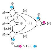
Figure 6.8: If stuttering actions are explicitly represented using Ø-labeled self-loops, then the livelock acceptance can be specified as visiting finitely many transitions not labeled by **1**.
