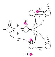
**Figure 4.8:** Converting the automaton of Figure 4.7 to use generalized Büchi acceptance, or in this case, Büchi acceptance.
