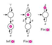
**Figure** 4.3: Three minimal automata for FG*a*, using: state-based Büchi acceptance, state-based co-Büchi acceptance, and transition-based co-Büchi acceptance.
