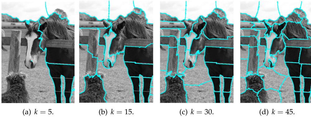
FIGURE 2.16: The segmenting results by using normalized cut algorithm with different value of number of segmentation k . The image is extracted from [160].
